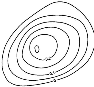
**Figure 9.6** Typical tiltmeter ground surface heave contour.
