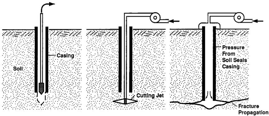
Figure 9.2 Method for creating hydraulic fractures in soil.
