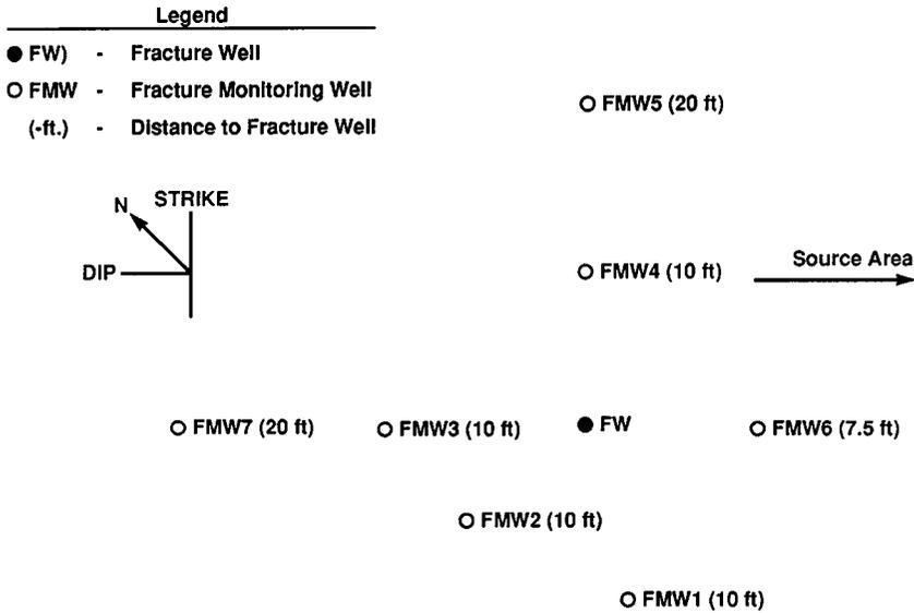
**Figure 9.8** Well location plan for pneumatic fracturing.
