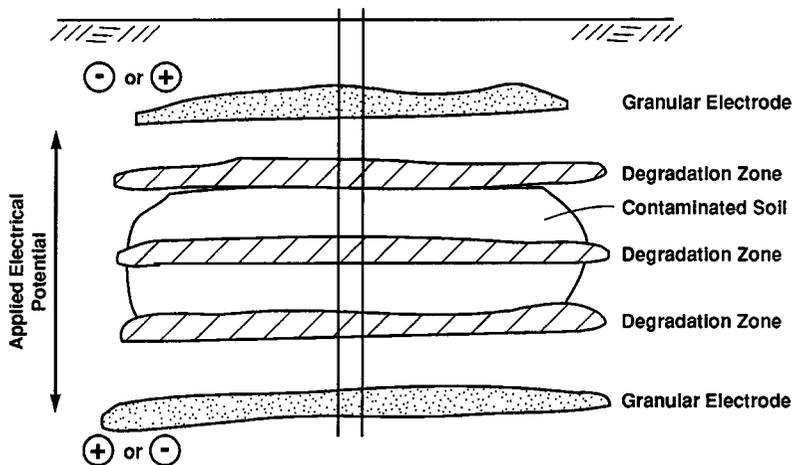
**Figure 9.10** Schematic diagram of the “lasagna process.”
