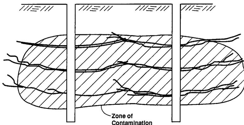
**Figure 9.7** Successive fracturing of target zone with overlapping fractures.
